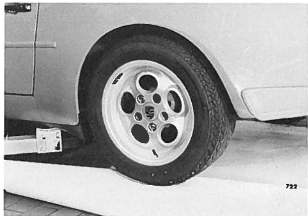
Rear Wheel Consisting of 8 J x 16 H 2 Rim and 225 / 50 VR 16 Tire
